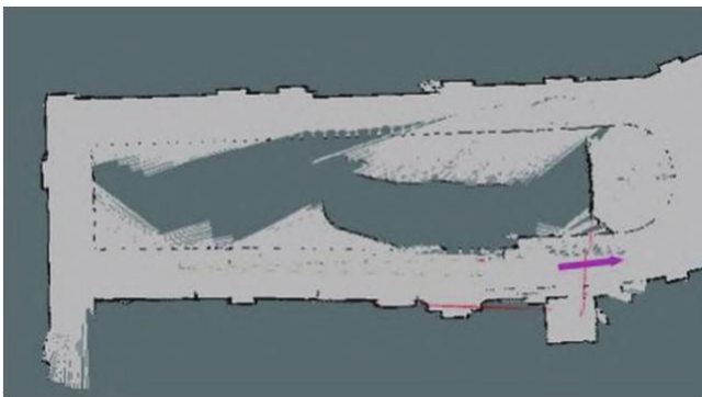
Figure 10. Path planning on the two-dimensional grid map of the sixth floor of Building 3
