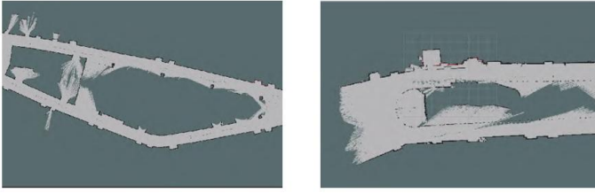
Figure 9. Two-dimensional grid map of the sixth floor of Building 3 constructed by the Cartographer-SLAM algorithm
